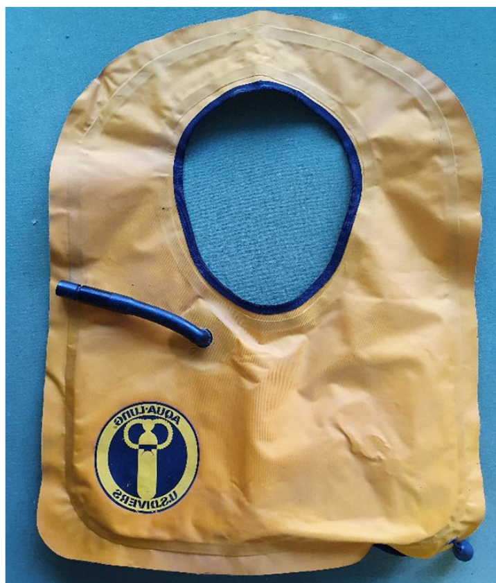
Figure 2. An early US Divers Safety Vest. The oral inflator is visible on the left. The CO2 cylinder is situated lower right at the back out of sight. The emergency pull cord is visible at the lower right of the vest.
