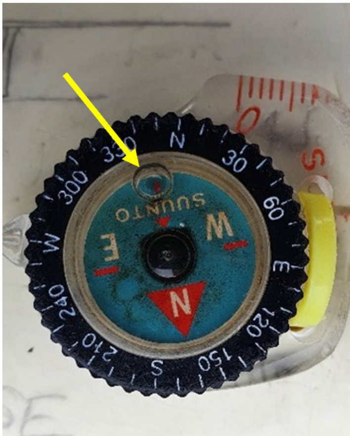
Figure 3. Photograph showing the bubble in the compass (arrow).
